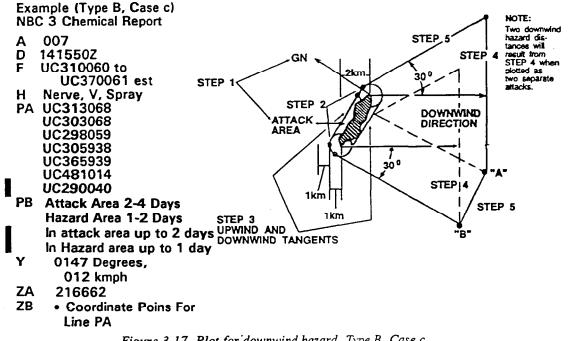
Figure 3-17. Plot for downwind hazard, Type B, Case c.
